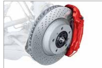
Standard brake system on the 911 Carrera S and Carrera 4S
