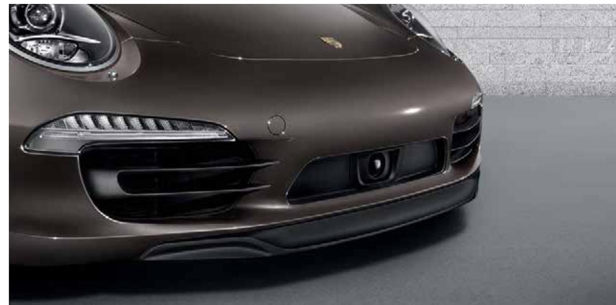
Radar sensor of Adaptive Cruise Control
