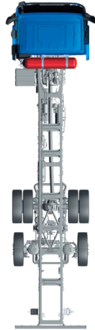
CNG tanks behind the cab, available in combination with: • Left side CNG; right side CNG • Left side CNG; right side free • Left side free; right side CNG
