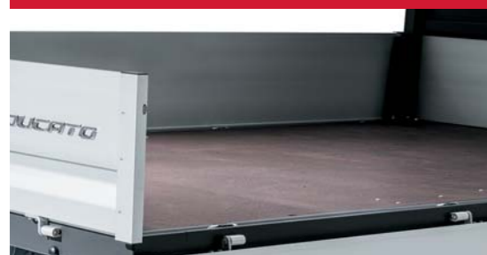
The load platform is lined with robust marine plywood.
