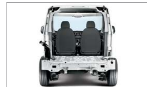
Anchorage points on the cab and platform, optimum setup for all types of body
