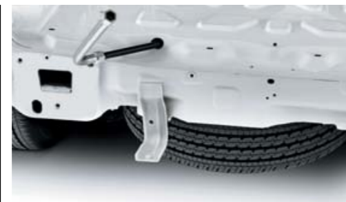
Spare wheel accessible from the rear and compatible with most bodies (opt. 980)
