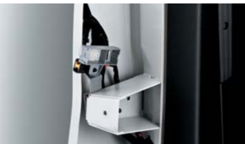
Transformer socket - electrical interface for connecting body equipment services (opt. 081)
