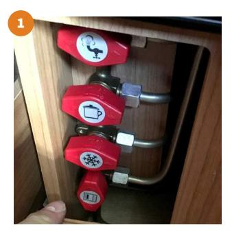
Open all tank drain valves to drain onboard and external tanks, and leave open.
