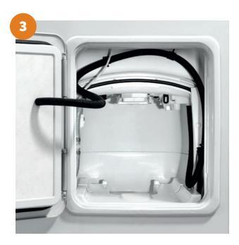
Empty the fresh water tank using the drain tube / fresh water tank level indicator. Pull the lever indicator / drain tube down from top plug position and outward through door opening to drain water from the tank then empty the water fill funnel by pulling the bottle away from tank.
