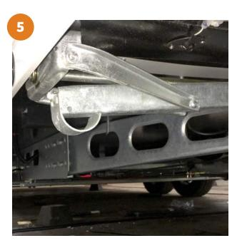
Lubricate relevant points on the chassis.
