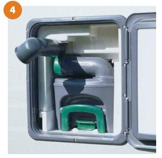
Remove the small water cap on the filler bottom, allowing water to drain from the water funnel. (Not C-200 toilet). Do not tighten caps, this helps in keeping unit dry. The pour out spout and vent plug can be removed. Seals should be greased if necessary with acid-free Vaseline.
