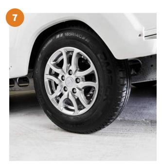
Or if being left on road wheels rotate wheels (every two weeks) and ensure the correct tyre pressures are maintained.
