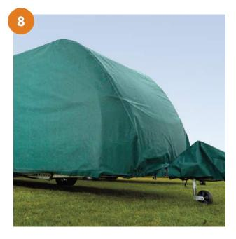
A purpose made cover maybe used, but please ensure the cover is a good fit, breathable and securely fitted.
