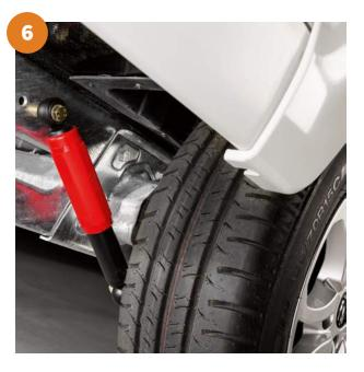
If not being left on road remove road wheels, using the correct jacking points and suitable axle stands.
