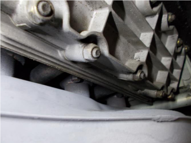
No leaks from cam covers
