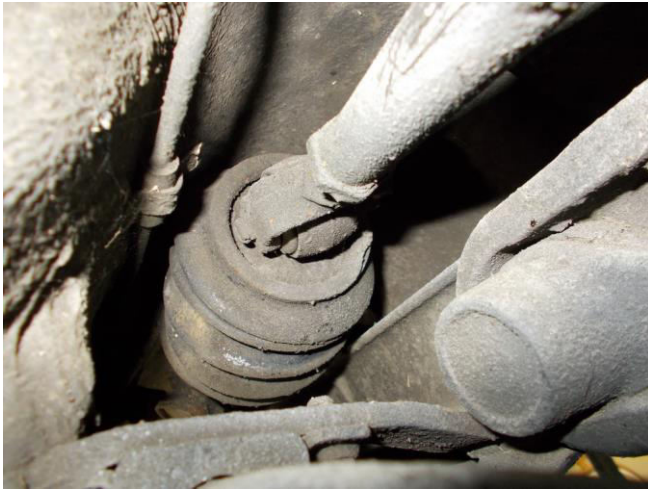
No leaks from front dampers
