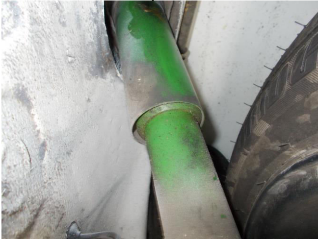
No leaks from front dampers
