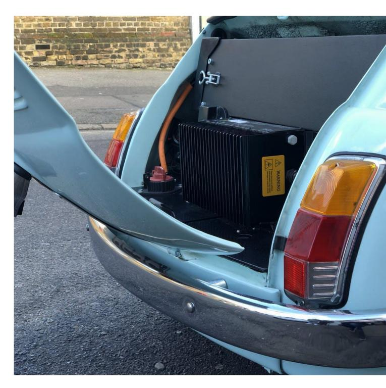
Yes, before you shake your head in disbelief, this tiny car packs a trio of Tesla batteries in its arsenal giving it 16kWh of juice, which is good for some 60-75 miles of range depending on driving style. Perfect for daily use in the vast urban sprawl. This setup takes a shade over seven hours to charge via a 1.5Kw charger. To complement this, there is an optional 2.5Kw charging system that completes the task in just over four hours.
