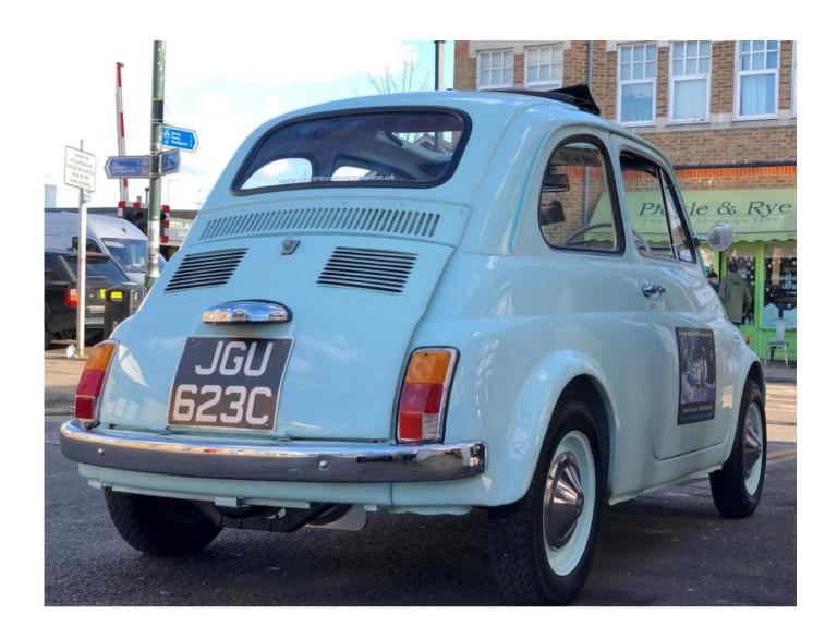
A majority (almost all) of EVs are equipped with a single speed gearbox due to the massive torque outputs involved. With the Electric 500 though, things get really smart as it retains its original four-speed manual box.
