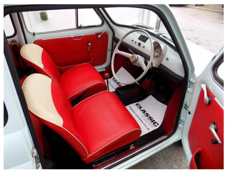
The only additions you will find in the cockpit are new controls for the electric heater in place of the original levers between the seats for the choke and starting the car.
